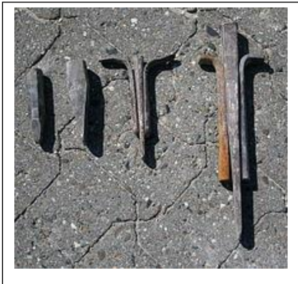
“Plugs and Feathers” (wedges for quarrying Portland Stone)
